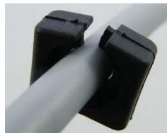
Apply rubber seals of the appropriate size (widest side up): the top edge should be flush with the housing. Fix the cable to the tab with cable ties, and cut off any protruding cable tie ends.
